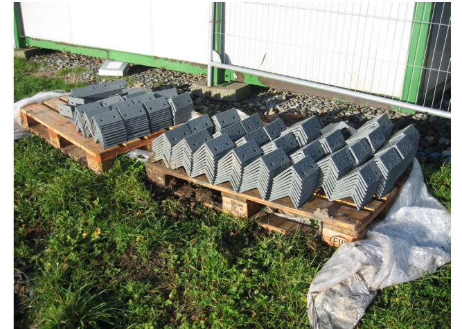
DfD steel cleats with pre drilled bolt holes.
