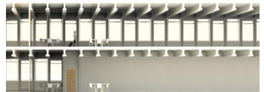
Section showing exposed structure
